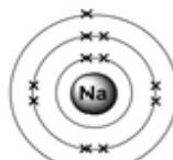
The electronic configuration of Sodium (Na) can also be written like this 2,8,1. This shows there is 2 electrons in the 1st shell, 8 electrons in the second shell and 1 electron in the 3rd shell.
